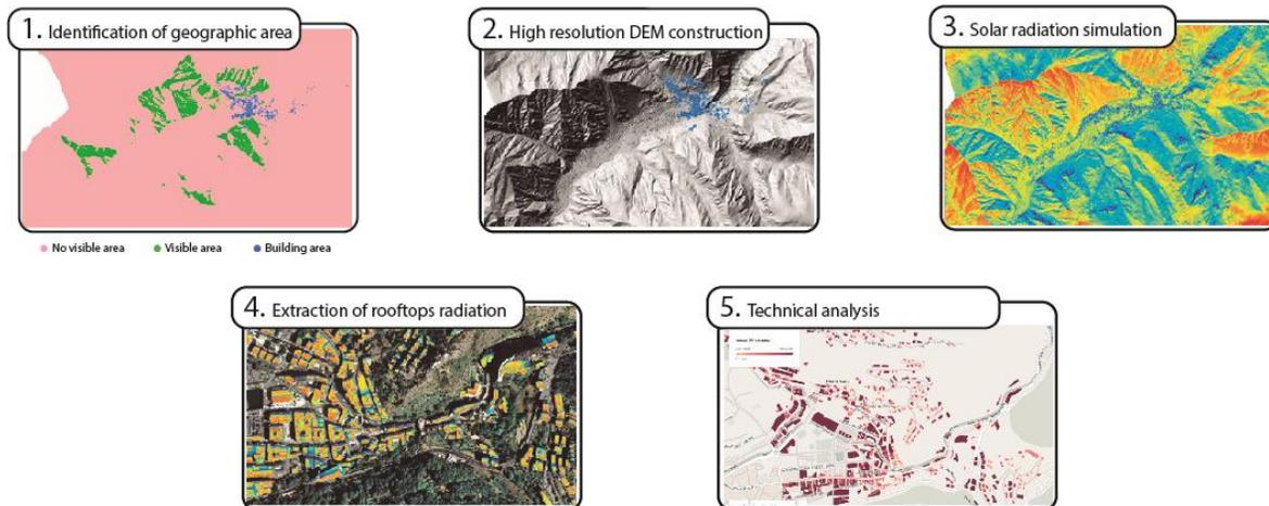
**Fig. 2.** Flowchart of the methodology to estimate rooftops PV potential
